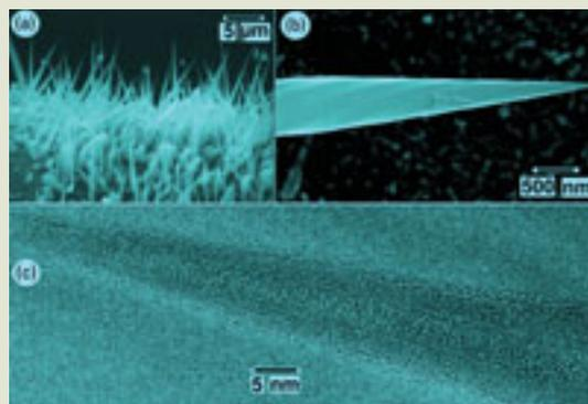
Microscopy images showing (a) aligned TGCs grown on an iron needle surface, (b) the faceted and helical appearance of a TGC, and (c) a TGC tip. (Adapted with permission. Copyright 2003 American Association for the Advancement of Science.)
