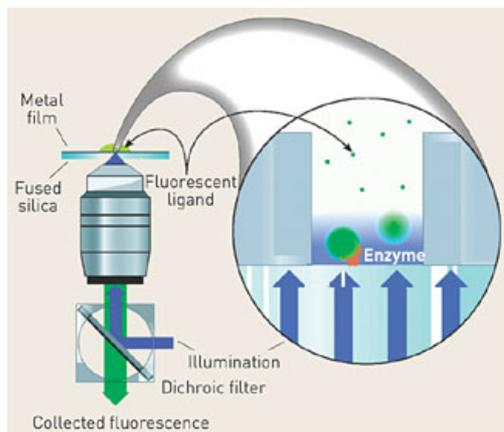
**SINGLE-MOLECULE DETECTOR** Webb, Craighead, and coworkers developed this "zero-mode waveguide" technique for detecting single-molecule phenomena. © *SCIENCE* 2003
