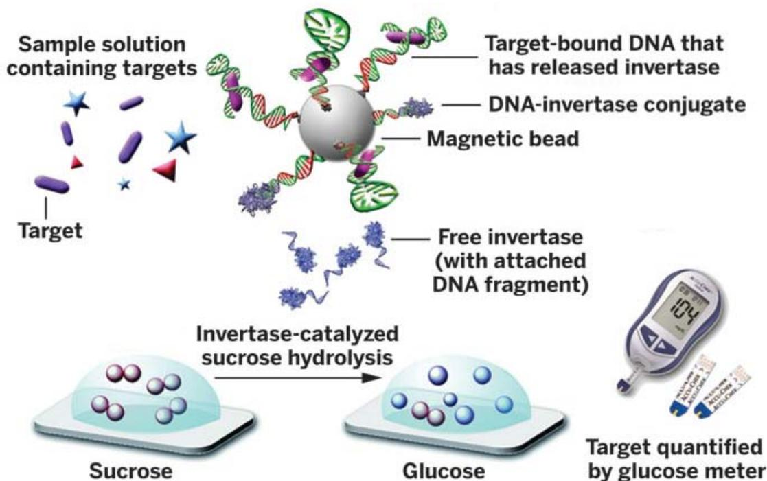
REPURPOSED Personal glucose monitors can measure invertase-catalyzed glucose production to quantify a target substance.
